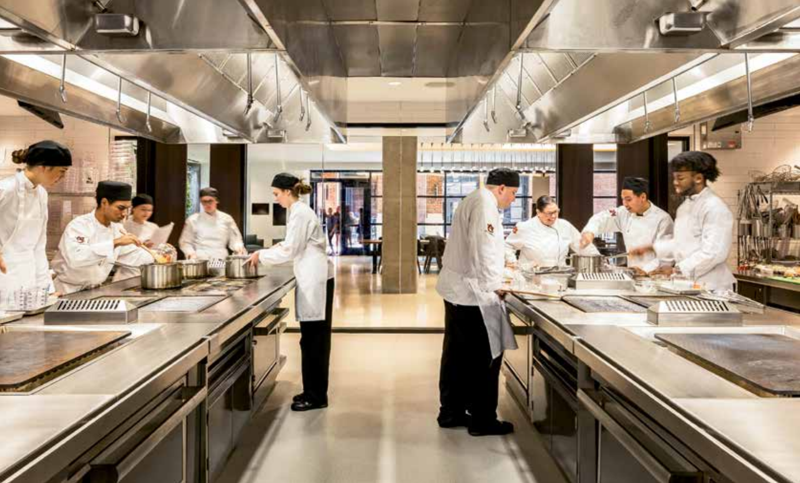
Above: Culinary Laboratory 1 contains two 20-quart mixers, two food processors, two blenders, two slicers, an induction cooker and a vacuum packing machine. A combi oven sits at the end of one of the dual cooking suites. Each cooking suite contains a six-burner range along with a chargrill, dual fryers, a flattop griddle, a plancha and a pasta cooker.
